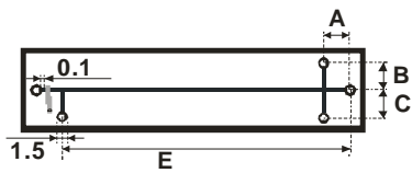
Fig. 14: Chip layout with electrode
