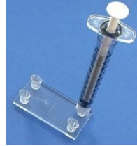
Fig. 21: Chip with Luer Lok compatible fittings (diameter of Luer Lok-through hole: 1.3 mm)
