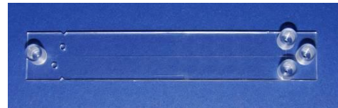
Fig. 10: Chip with integrated fluidic reservoirs
