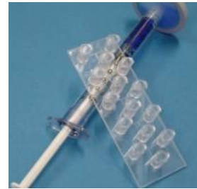
Fig. 21: Schematic drawing of the adapter Fig. 22 & Fig. 23: Luer Lok compatible adapter
