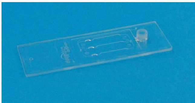
Fig. 30: Platform for the development of diagnostic assays involving whole blood like agglutination assays. The chip contains Luer-connectors and three identical fluid pathways leading to antibody-filled reaction chambers.
