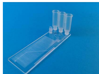
Fig. 27: Tanks mounted on chip
