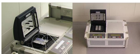
Fig. 43: The thermal control unit with two triplets of individually controllable temperature zones.
