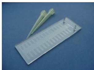
Fig. 42: 15-cycle continuous-flow PCR chip
