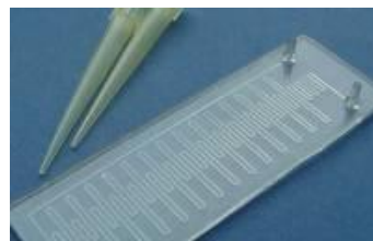
Fig. 36: Use of the 2-olive platform for a continuous-flow PCR chip
