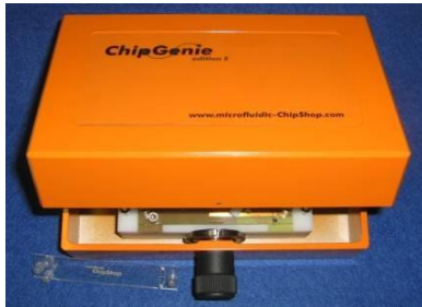
Fig. 47: ChipGenie® edition E capillary electrophoresis unit
