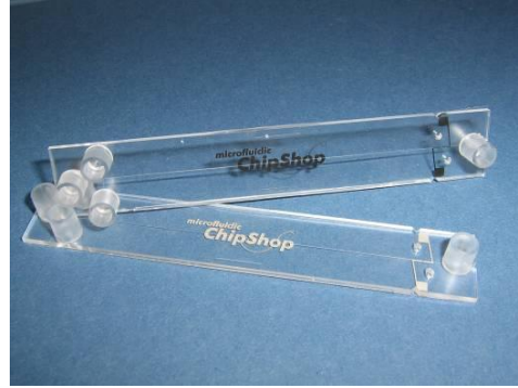
Fig. 17: Actual image of the CE-chip with screen-printed electrodes
