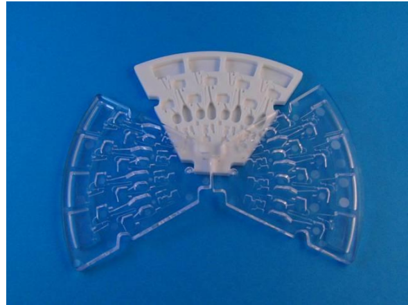
Fig. 20: Example of actual chips in transparent and white materials
